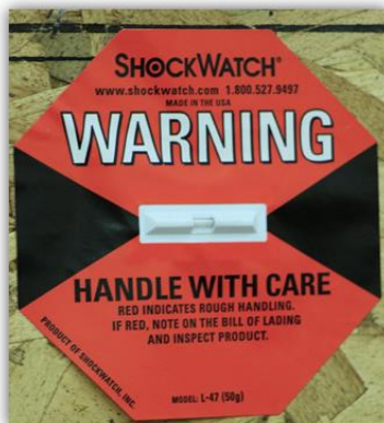
Accelerometer to measure the g-force
