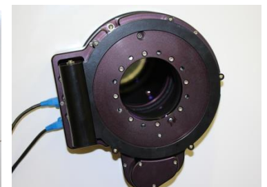
Rotator-focuser system (Nasmyth Port) for attaching the instrumentation.
