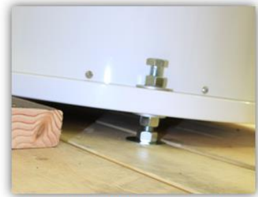
Bolts and wood holding telescope off the platform
